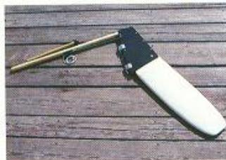
Every O'Day daysailer has a kick-up rudder for shallow draft sailing and added safety when beaching or hauling the boat.
