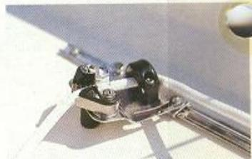
Jib sheets are adjustable on all daysailers from O'Day. Cockpit floors and all decks have molded-in anti-skid patterns.
