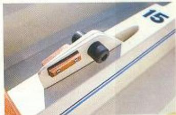
Adjustable centerboards and daggerboards are standard for shallow water sailing and improved performance on and off the wind.
