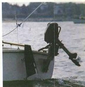
All O'Day daysailers are designed and built so that outboard motors can be easily and securely mounted. (An extra-cost optional bracket is needed on the O'Day 19 only.)
