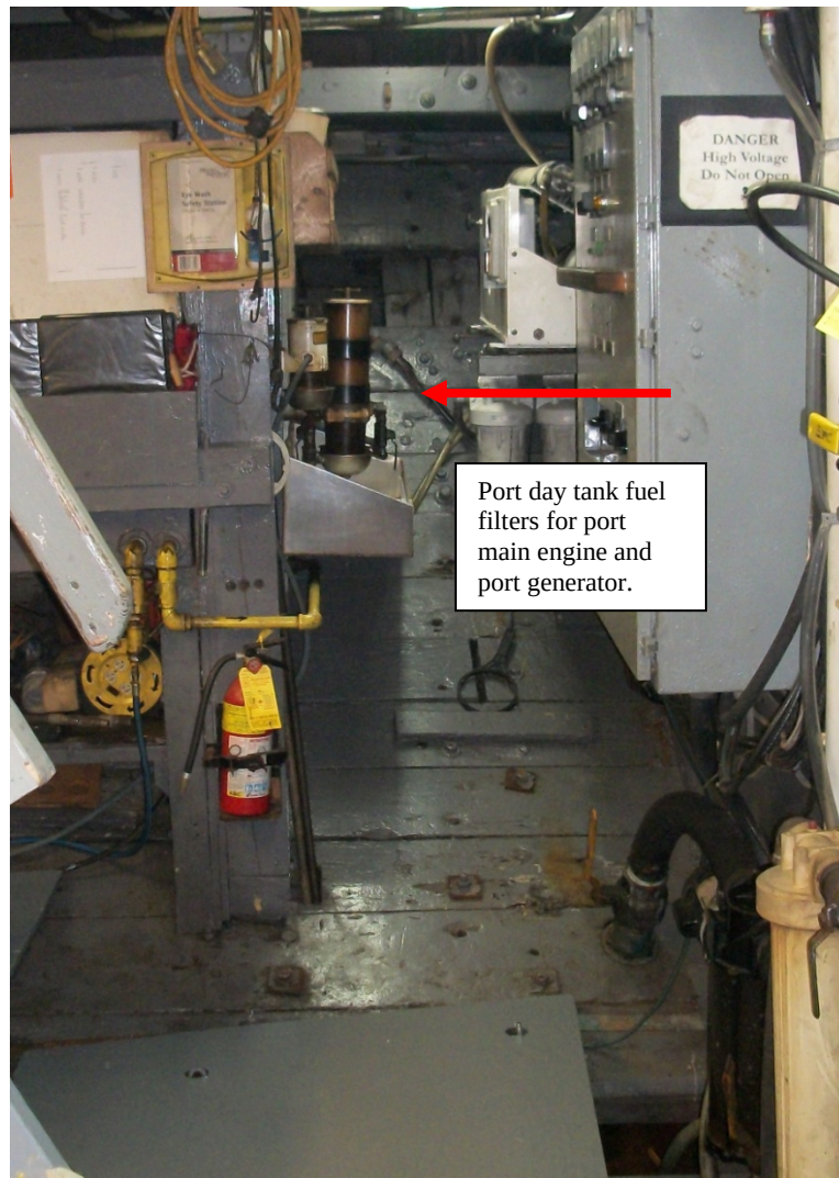
Figure 5 BOUNTY's port day tank and fuel filters.
