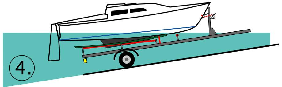
Notice bow making contact with bow roller and lifting bow up and sinking the stern
