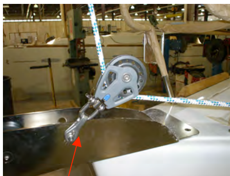
Tack block shackled to toggle on bow roller
