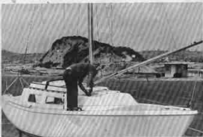
Step 23 —Connect forward shrouds. Disconnect and remove stabilizer. Release tension on sheetline and remove ginpole from mast. Disconnect jib halyard and return it to mast.
