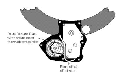
When the motor solder joints are made, fit a tie wrap around the Mu metal shield and the Black and Red wires to retain shield and wires.
