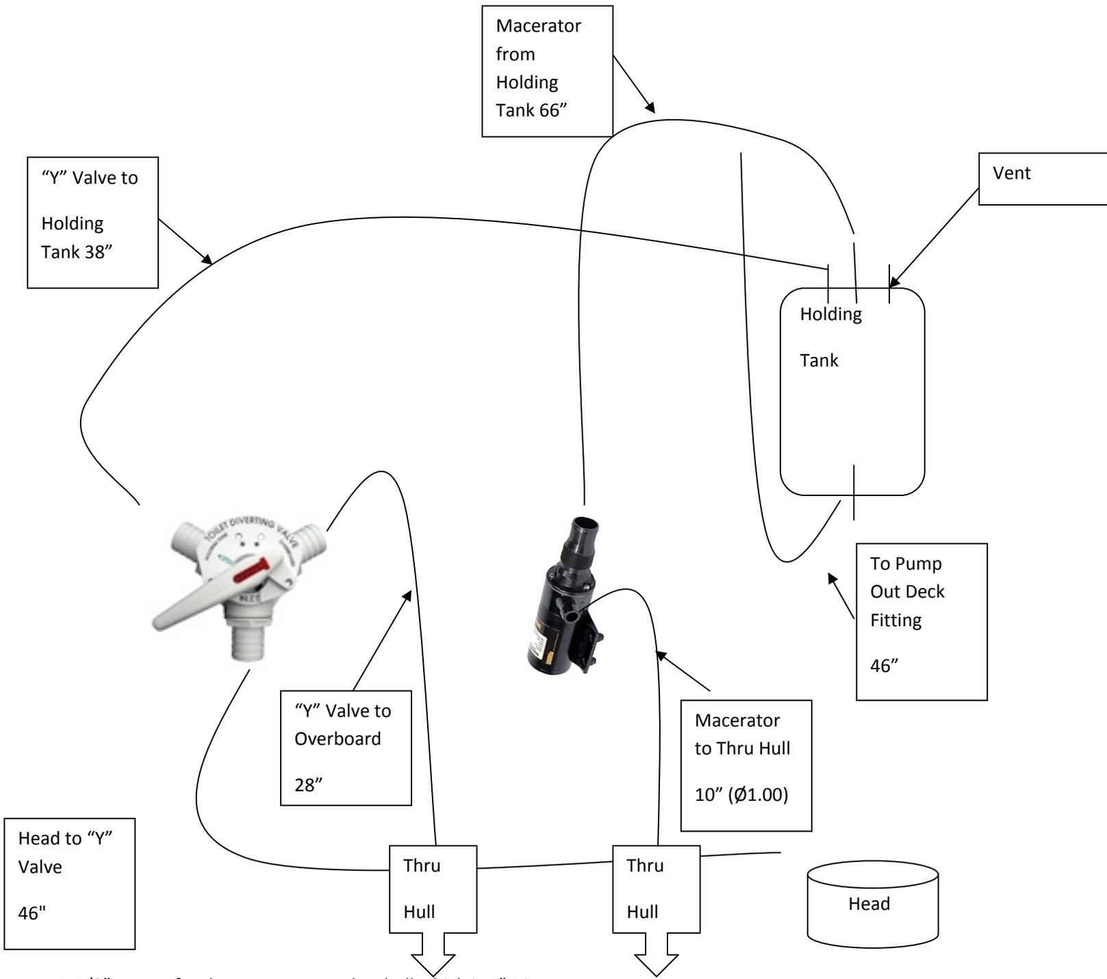
All hoses are 1-1/2" except for the macerator to thru hull which is 1" Diameter.
