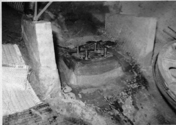
The upper bearing, above left, was a plastic bushing in a wooden block and was getting worn. Jim fabricated a new one out of Delrin sandwiched between aluminum plates, above right. Jim glassed the block for the lower bearing to the hull after aligning it with a pipe, at left, then assembled the bearing and shaft seal to it using 3M 5200 as the sealant, below left. Once everything was back together, Jim's steering system was as good as new, or even better in parts, below.
