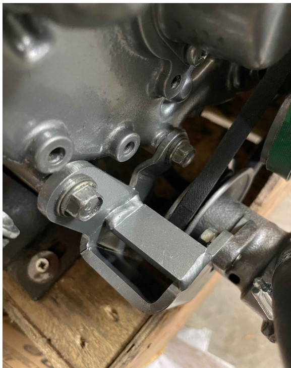
Back bracket offset to timing cover case
