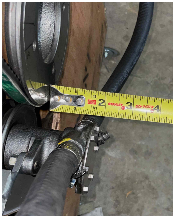
Rotated pump requires 2" in front of pulley
