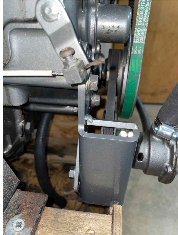
Pump alignment on new YM series bracket mounted directly to the timing case.
