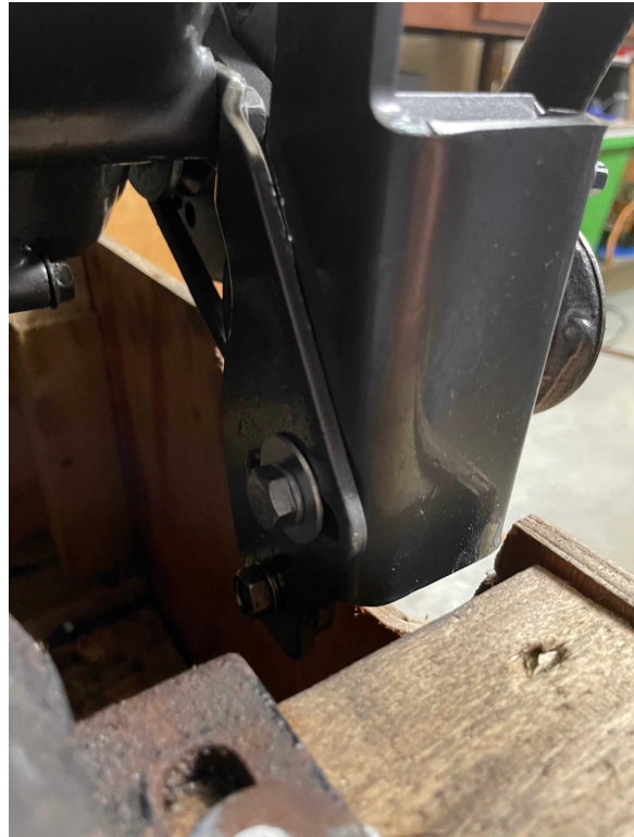
Strongback bracket mounted on YM bracket with 2 points of attachment. I also found it necessary to enlarge the upper slotted hole to allow enough movement for adjustment
