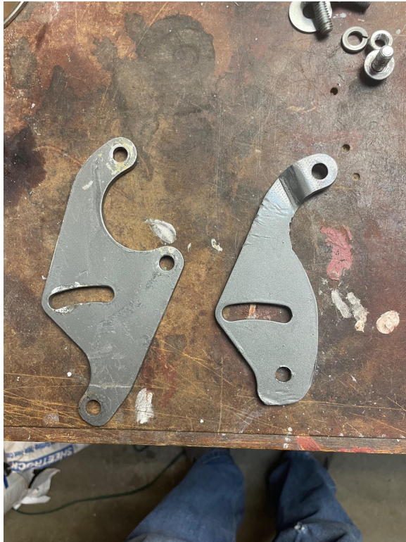
Modifications to original bracket to serve as strongback bracket for YM bracket
