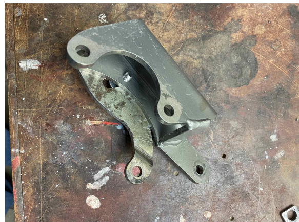
Back bracket mounted on YM bracket
