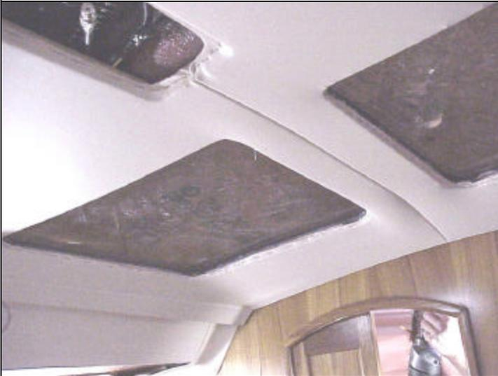
Headliner ready for trim rings. Whisper is stapled to the inside of the wood not the bottom.
