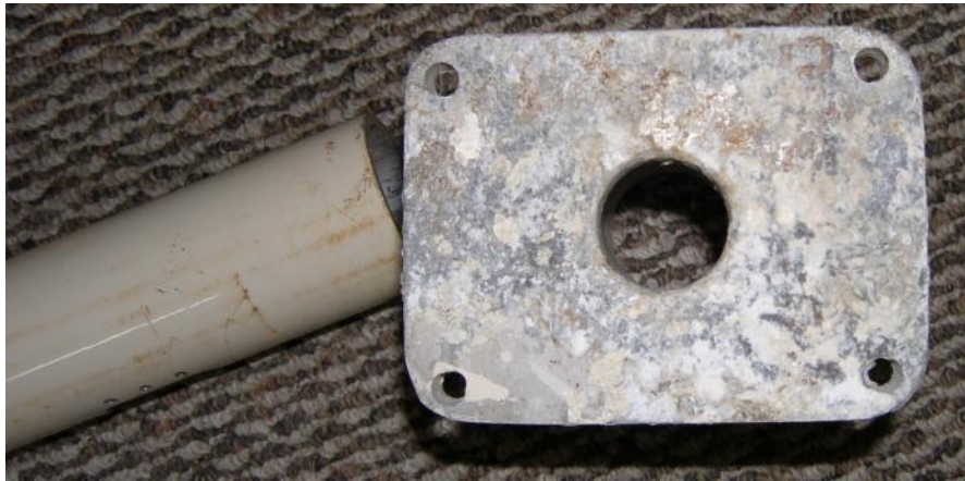
Top of compression post upper foot. Mast wiring enters through opening in top of flange and exits via the side opening. Post OD is 2 7/8-in and ID is 2.5-inch AL.
