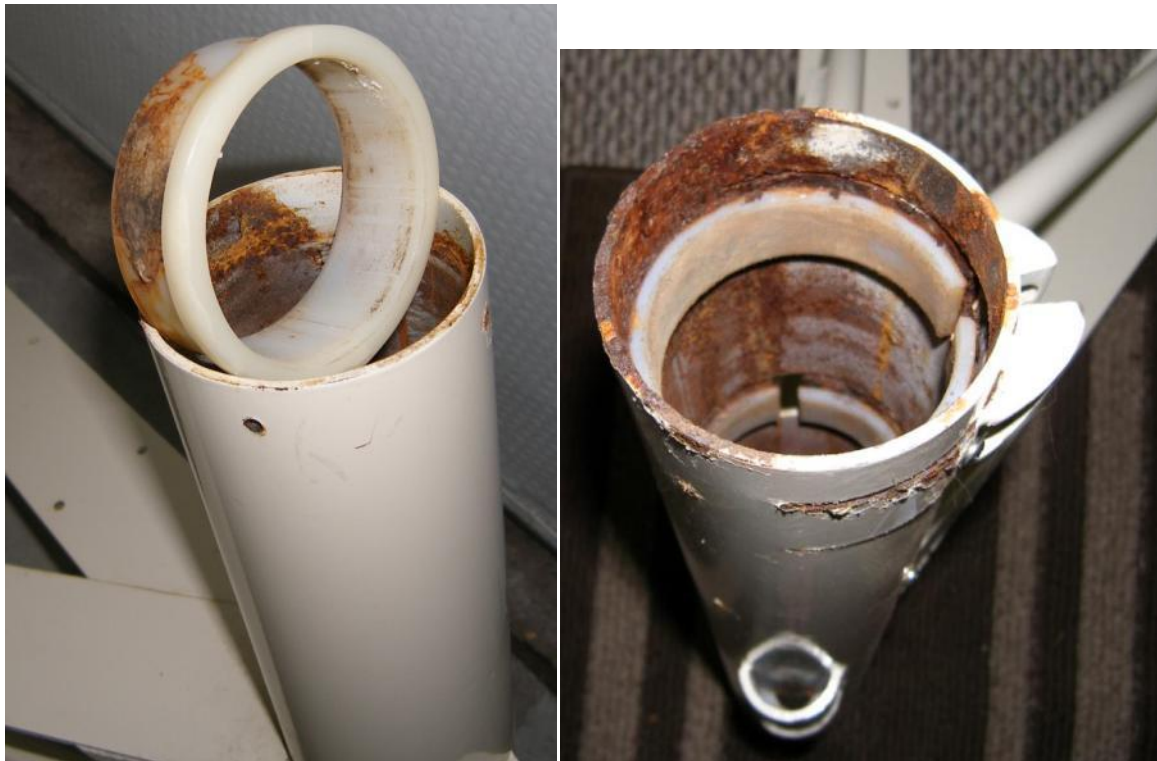
Upper nylon insert removed (left). It the inner nylon/plastic surface was actually flaking off. Bottom view of sleeve (right) showing lower two internal nylon slides. The rust on the inside of the sleeve actually compressed the nylon inserts to become an interference fit with the compression post.
