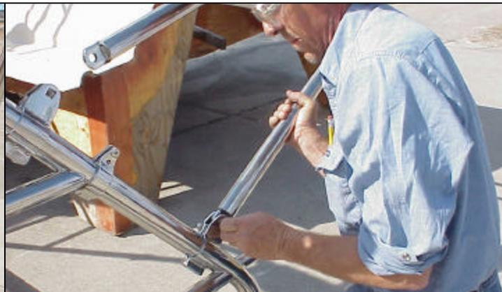
Using two people put the lower legs of the davit main frame into the lower clamps on the arch. Insert a 1/2-13 x 1-3/4" stainless steel carriage bolt thru the clamp and davit so the head is outboard (unless the owner wants the bolts to face outboard). Put a 1/2" stainless steel lock washer & 1/2-13 stainless steel nylon insert lock nut on the carriage bolt, do not tighten yet.
