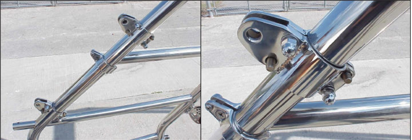
Mount the four stainless steel clamps onto the arch as shown, two on each side. The bolts should be facing in-board, if owner prefers the system can be attached with the bolts facing outboard. Place two lock washers & acorn nuts on the clamps as shown then loosely tighten them by hand.
