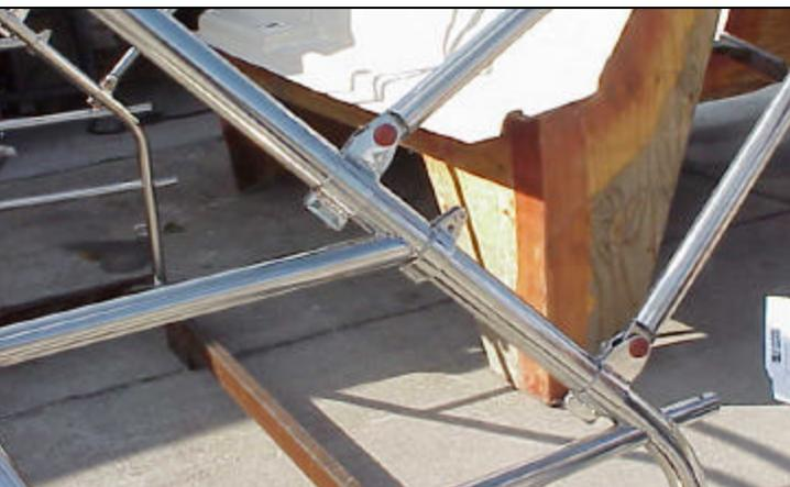
Rotate the davit main frame up and attach the upper legs of the davit into the upper clamps in the same manner as before. NOTE: Carriage bolts on right picture are painted for clarity only.
