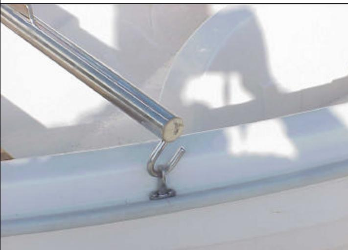
The other end of the block and tackle assembly will attach to the extension frames as shown. The upright end on the extension frame will be towards the mother vessel. The longer extension goes to the starboard side.
